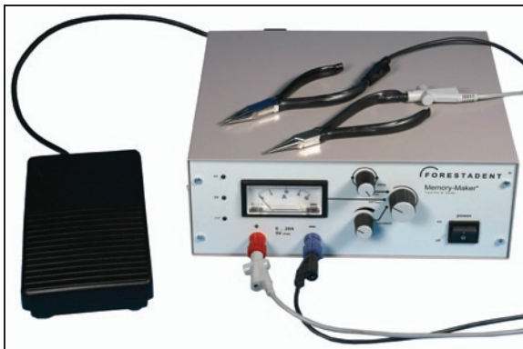
Fig. 1 Memory-Maker with two electrically connected pliers and rectangular foot switch.
